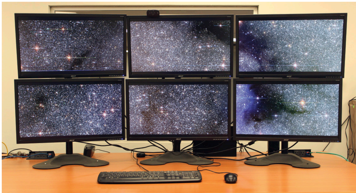
Figure 2: Color images constructed from a single raw exposure in each of i , z , and Y filters as per Figure 1—this time from six detectors within the DECam field of view—displayed on the 2 \times 3 array of monitors at one of the observer workstations in the Blanco control room. This figure shows 10% of the 60-chip field of view of DECam. This image is centered near (l,b)J2000.0 = (7.11^\circ, -1.63^\circ) . (Image credit: Will Clarkson, Kathy Vivas, R. Michael Rich, and the BDBS collaboration.)
