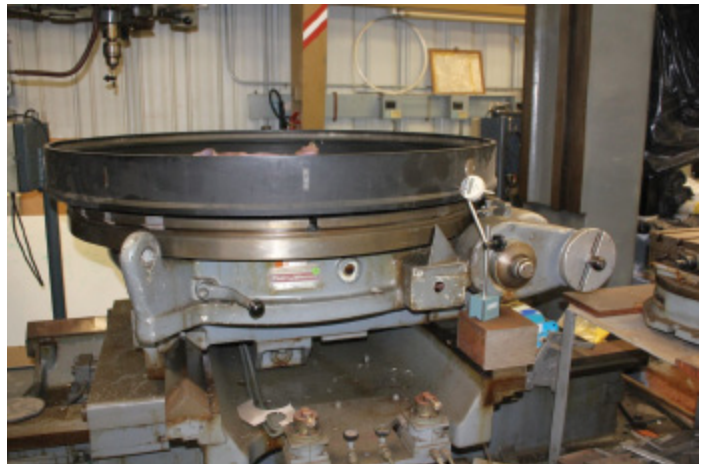
Figure 6: Checking the mirror cell for distortions and other damage; none were found.
