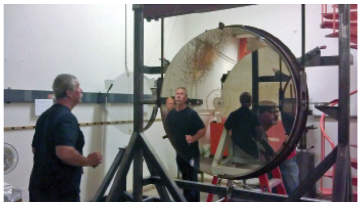
Figure 2: Preparing for optical tests. The mirror is lifted off its handling cart (top) by Ron Harris (left) and Gary Poczulp (behind the mirror) and installed on its test fixture in the basement of the NOAO optics shop (bottom). In this bottom photo, Gary is on the left (and twice in reflection) and Joe De Vries is seen behind him in reflection.
