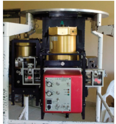
Figure 6: A two-channel infrared photometer used on Cerro Tololo in the 1980s.
