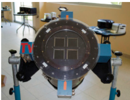
Figure 5: The Big Throughput Camera (BTC), the first optical imager with a detector mosaic of four CCDs. The BTC was installed on the Blanco 4-m telescope in 1996.
