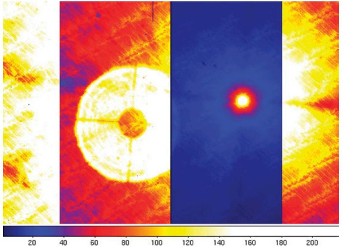
Figure 1: The laser spot imaged with SOI. The SOAR telescope was focused to 7 km to have an in-focus laser spot. Next to the laser spot is an out-of-focus image of a bright star.
