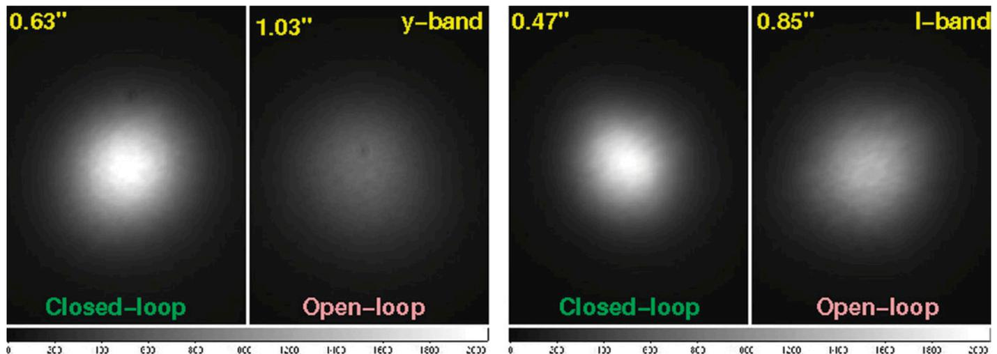
Figure 2: 16 April 2011. The loop was closed on the laser guide star on April 15. The next night the improvement of the image quality in closed-loop was documented by images of bright stars. Side-by-side comparison of point spread functions in the green and red are shown in the image, with full width half-maximum indicated.
