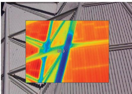
Figure 2: Thermal picture of the ice plug in cracked column. (Image credit: W. Goble, NOAO/AURA/NSF.)
