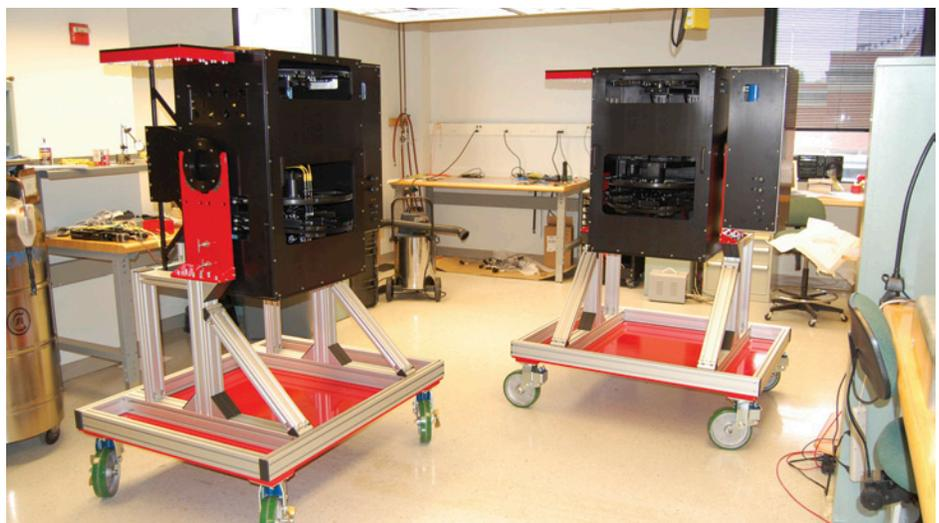
Figure 2: KOSMOS (right) and COSMOS (left) in the final stages of electrical and mechanical integration at The Ohio State University in Columbus, Ohio. The spectrographs are shown on their handling carts in the up-looking position, which is the same way they will mount in the cass cages of the 4-m telescopes using an adapter that is not shown. The Dewars install on the bottom of the instruments. Various covers are not yet installed in these photos.
