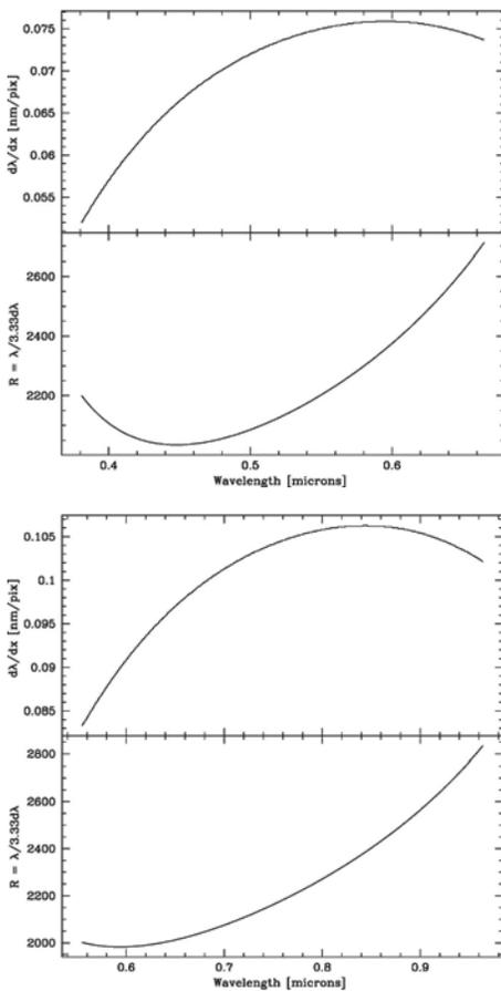
Figure 1: Dispersion curves for the blue (top) and red (bottom) gratings. The resolution shown is specified for a 1-arcsec slit, but the slits that will be provided will actually be 0.6, 0.9, 1.2, and 1.8 arcsec wide, plus a wider slit for photometric calibrations. The instrument image quality should allow use of the 0.6-arcsec slit for those willing to accept the associated light losses at the slit.
