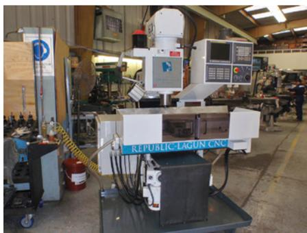
Figure 8: New Computer Numerical Control (CNC) machine for the La Serena shop. (Image credit: Enrique Figueroa, NOAO/AURA/NSF.)
