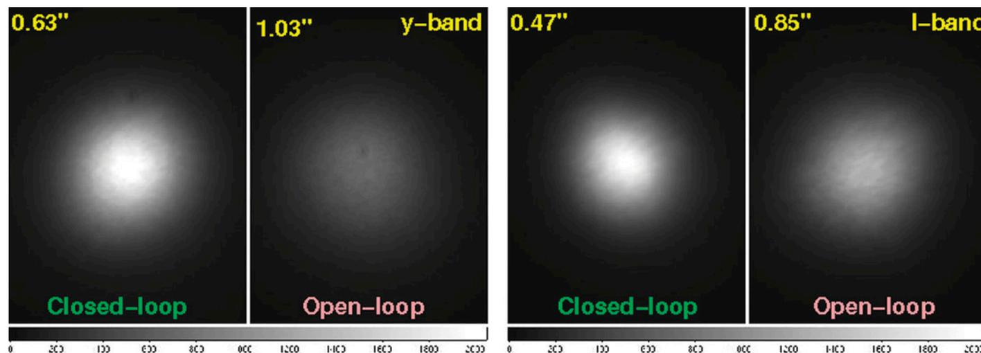
Figure 2: 16 April 2011. The loop was closed on the laser guide star on April 15. The next night the improvement of the image quality in closed-loop was documented by images of bright stars. Side-by-side comparison of point spread functions in the green and red are shown in the image, with full width half-maximum indicated.
