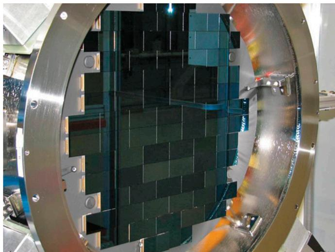
Figure 1: The Dark Energy Camera (DECam) focal plane with all 74 science-grade CCDs installed. On the Blanco Telescope, the 45 cm diameter focal plane covers 3 square degrees of sky, (12 times the area of the Full Moon). The fully depleted back-illuminated CCDs were made at LBL and packaged, tested, and installed at Fermilab. (Image credit: Juan Estrada, Fermilab).
