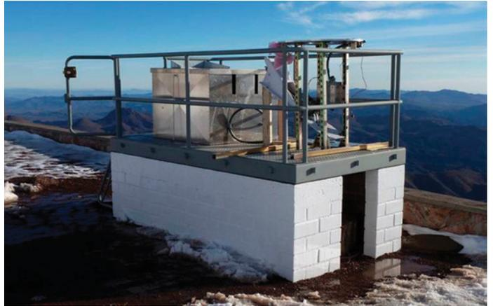
Figure 2: Radiometric All Sky Infrared Camera (RASICAM), built at SLAC by Peter Lewis and Howard Rogers under the supervision of Rafe Schindler, and installed at CTIO. (Image credit: Alistair Walker, NOAO/AURA/NSF.)
