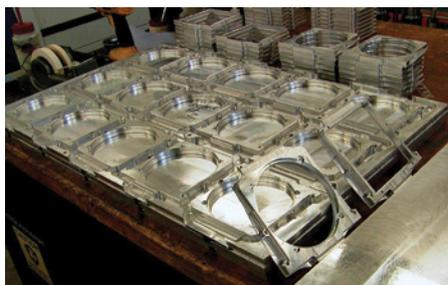
Figure 16: (left) New CNC machine installed in the Tucson shop. This machine already has seen significant use fabricating parts for the One Degree Imager (ODI) and ReSTAR Phase 1 COSMOS and KOSMOS spectrographs. (right) KOSMOS and COSMOS slit and filter wheel cells produced by the new Hurco CNC machine in the Tucson shop. (KOSMOS will be deployed in the fall of 2011 on the Mayall 4-m.) (Image credit: Roger Repp, NOAO/AURA/NSF.)
