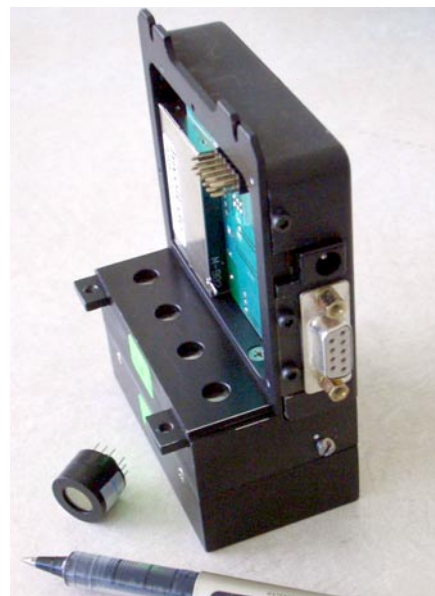
Figure 2. MASS-DIMM installed on a Meade LX200 telescope (left) and its electronics module (right) containing four tiny photomultipliers (one shown apart), photon-counting circuits, and microprocessors.
