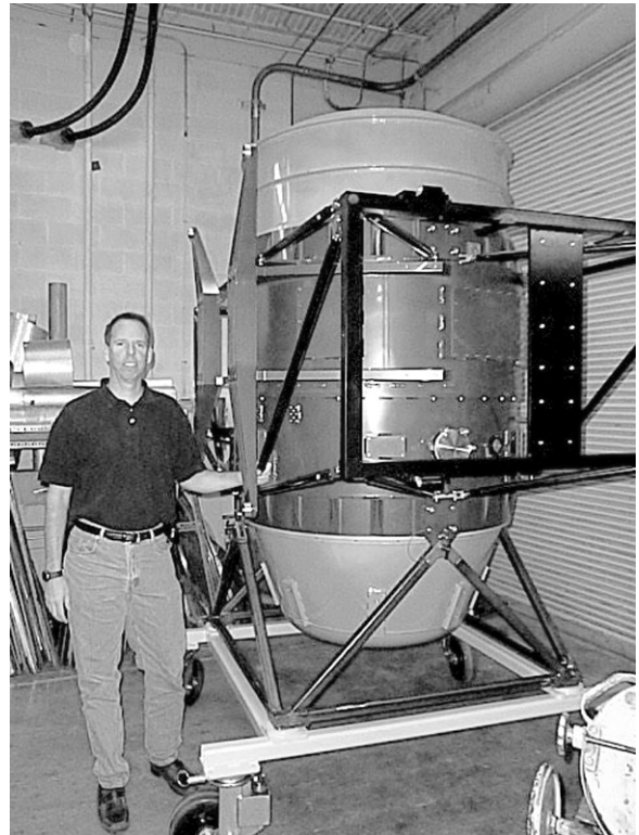
Senior Engineer Gary Muller is shown with the fully assembled GNIRS bulkheads and dewar shells, which were delivered to NOAO in December.
