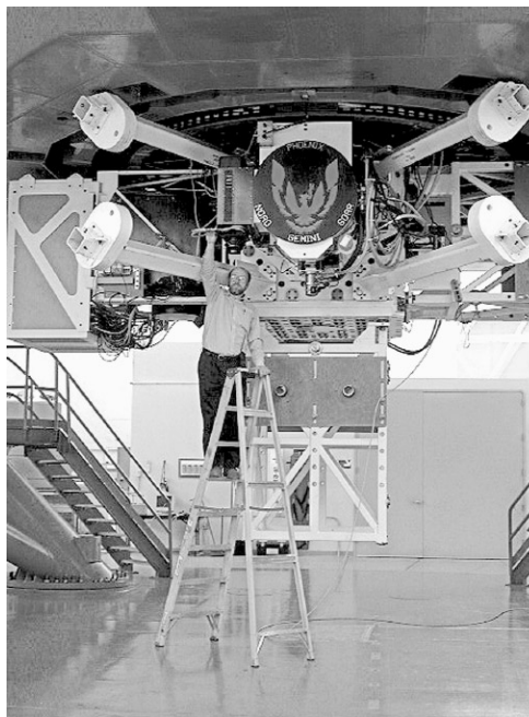
Phoenix is shown mounted to Gemini South, with Dr. Ken Hinkle standing on ladder under the telescope. The four "legs" are balance weights, required to bring the mass and center of gravity to within the Gemini specifications.
