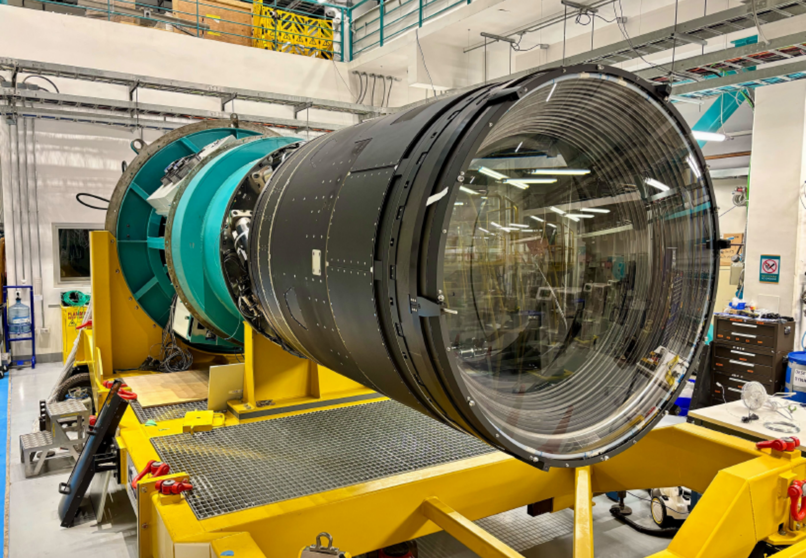
Figure 2: The LSST Camera mounted on the transportation cart (yellow) and installed on the integrating structure (teal). Looking from the lens toward the back, the hexapods that hold the camera to the rotator are visible behind the camera body, then comes the rotator itself, and finally the bulkhead plate that attaches the assembly to the telescope. The camera is parked in this view on level 3 in front of the white room. The lens cap is off of the 1.6 m first lens (L1), and one can see the shutter is closed. Credit: RubinObs/NOIRLab/SLAC/NSF/DOE/AURA
