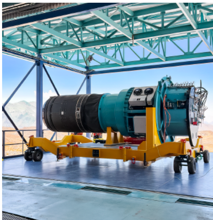
Figure 4: LSSTCam arrives at Level 8 (observing floor) on the vertical platform lift. The lift roof raises up, exposing the lift to daylight, when the lift reaches Level 8. The lift also provides a stunning view of the Chilean Andes on a typically clear and calm day. Credit: RubinObs/NOIRLab/SLAC/NSF/DOE/AURA
