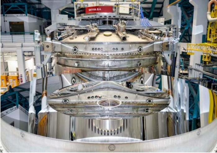
Figure 2: The freshly coated M1M3 mirror on level three and in front of its coating chamber. The telescope has a three mirror design. M1 (primary) and M3 are built on the same glass casting but have notably different curvatures. M2 is mounted at the top of the telescope, facing down toward M1. *Credit: RubinObs/NOIRLab/SLAC/NSF/DOE/AURA/T. Vučina*
