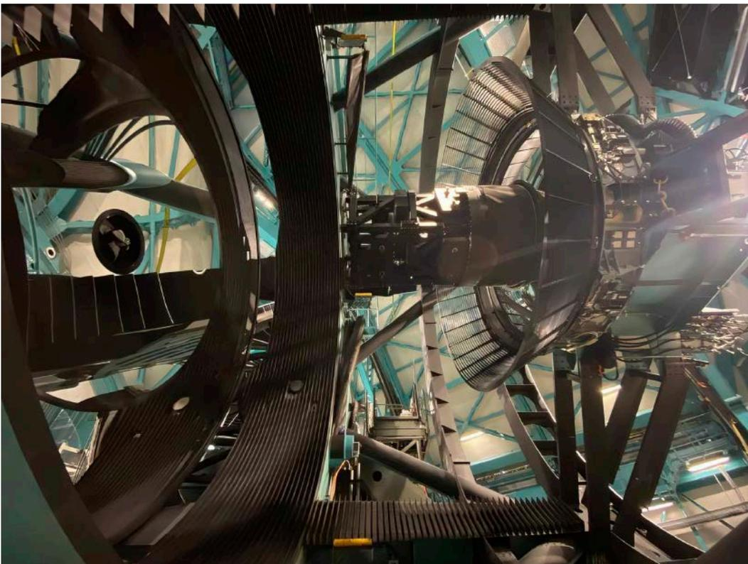
Figure 8: Parting shot, the fully functional system pointed at horizon. **From left to right**, M1M3, ComCam, M2 light baffle, M2 mirror and mirror cell. The central hole in M1M3 allows for cleaning and stripping chemicals to be captured and removed and provides access to the volume above the mirror when it is installed. Visible in the picture is a laser tracker mounted in the central hole that is used to align the telescope optics and camera. *Credit: Rubin Obs/AURA/NSF/B. Blum*
