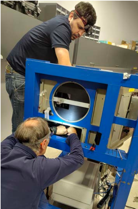
Figure 2: Tarcio Vieira and Andrei Tokovinin at the SOAR Telescope optics lab, installing cables inside SAM for the new deformable mirror
