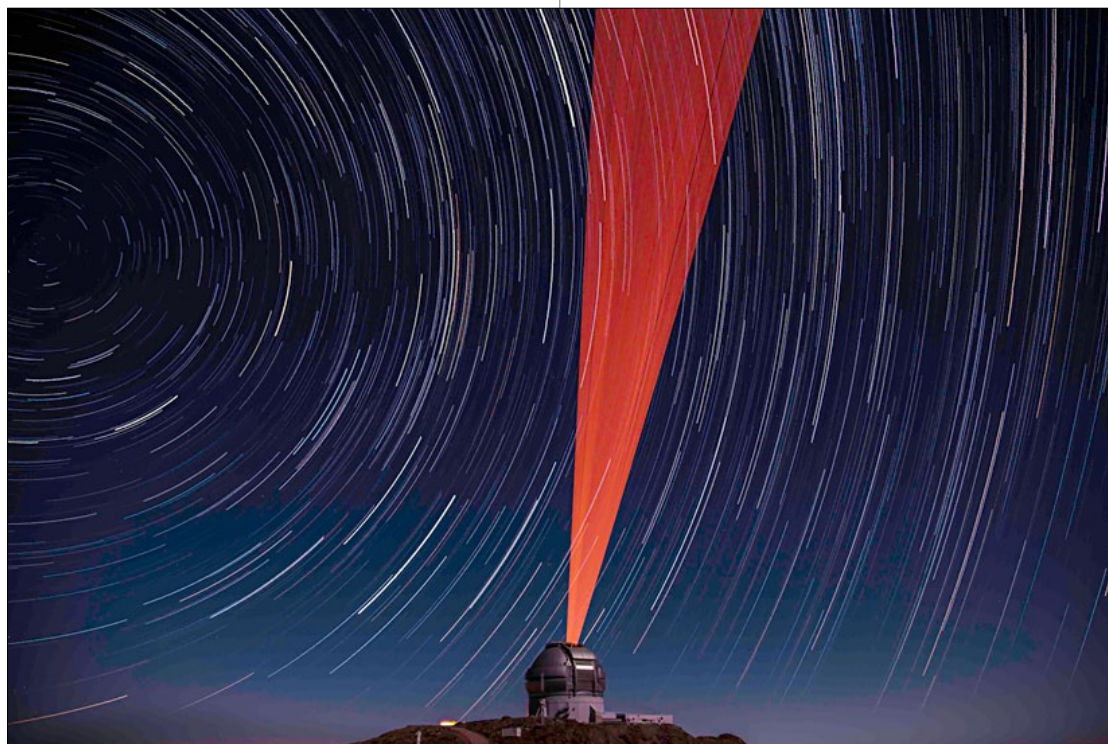
Figure 2: Gemini South laser propagates into the sky over Cerro Pachón. Despite lower power, many programs were successfully fulfilled due to the seasonal variations in the atmospheric sodium layer which provided stronger guide star returns.
