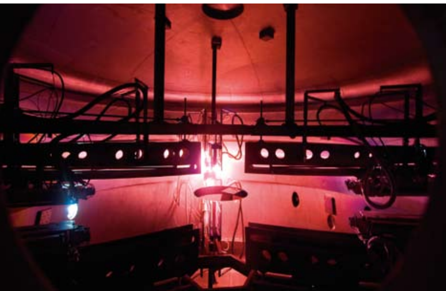
Figure 1. Magnetron three applying the very thin protective coating of silicon on top of the silver coated primary mirror.
