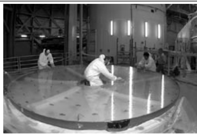
Figure 1: The SOAR primary mirror is meticulously cleaned at Gemini South prior to placement in the coating chamber.
