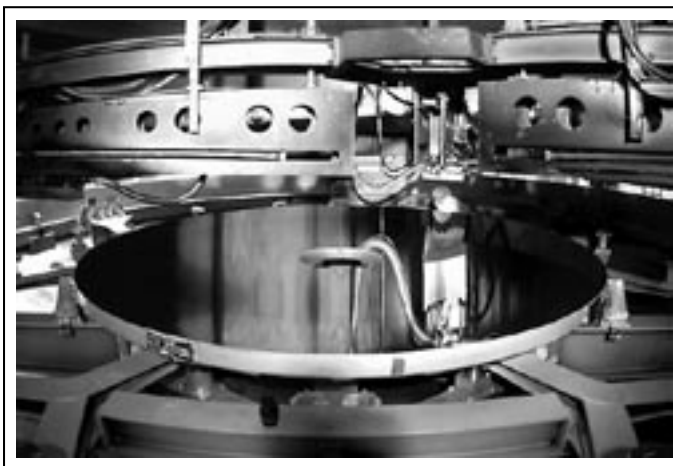
Figure 2: The freshly coated SOAR primary mirror seen inside the coating chamber at Gemini South.
