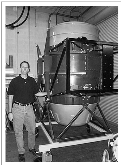
NOAO Senior Engineer Gary Muller is shown with the fully assembled GNIRS bulkheads and dewar shells, which were delivered to NOAO in December, 2001.
