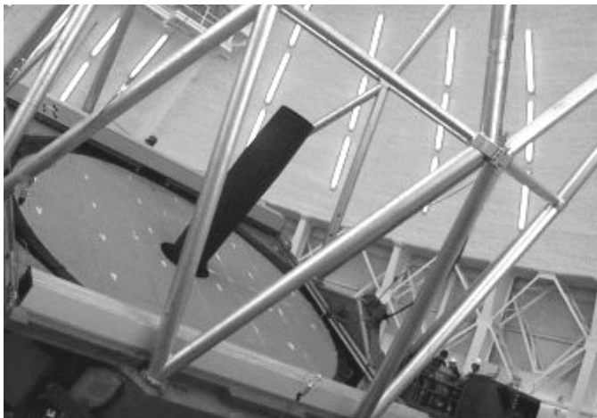
Figure 3: Cerro Pachón telescope with dummy mirror and pressure, wind, and accelerometer sensors.
