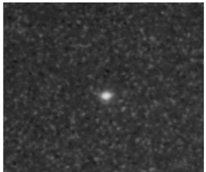
Figure 7: Image of star projected on viewing screen at Gemini South taken with the alignment telescope, a commercial camera, and the uncoated M1.
