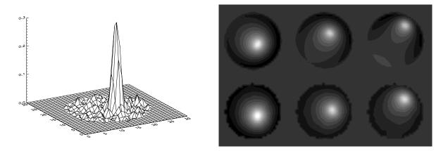
Figure 2. Left: Laplacian of the measured influence function for the electrode number 5. Right: The calculated (top row) and measured (bottom row) response of DM-79 for electrodes number 5, 16, and 48. All functions are displayed on the same intensity scale, the pupil diameter on DM is 38 mm. Tip, tilt, and piston are subtracted.
