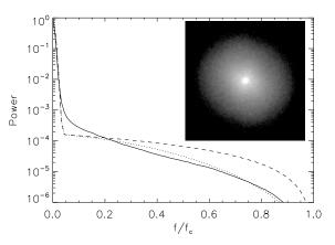
Fig. 2.— Power spectrum of the single star HR 1338 is radially averaged and plotted in full line in comparison with the model (1) with  $D/r_0 =$ 50.8 (dashed line). The dotted line is the same model with additional Gaussian blur of 13 mas rms. The insert shows the 2-dimensional spectrum with logarithmic intensity scale in the range  $10^{-6}$ to  $10^{-3}$ .
