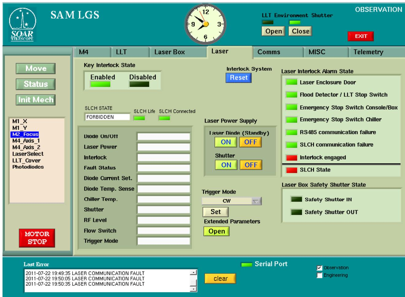
Fig. 3. LGS GUI with laser tab opened.
