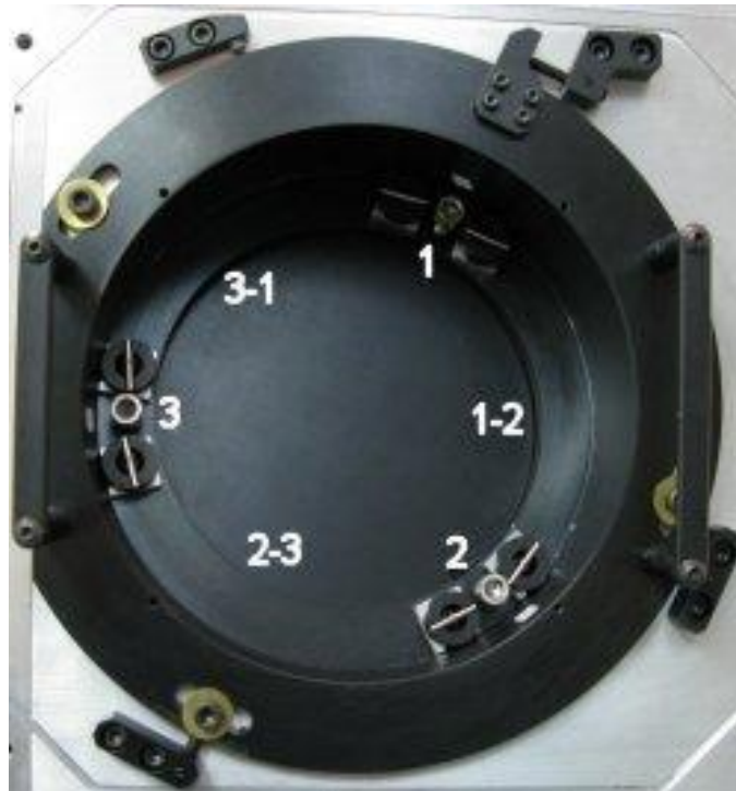
The OAP1 mirror mount aligned position
