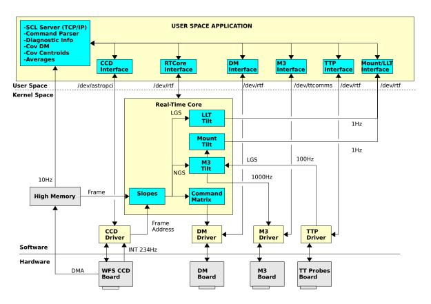
Figure 1.1: Block diagram of the Real-Time Computer Software
