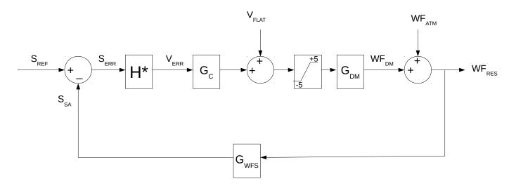
Figure 2.1: The WFS measures the residual wavefront slopes. The residual wavefront is projected to the DM actuators voltage space to be filtered by the controller. The resulting voltages are added to the nominal operation point voltages and then applied to the DM.
