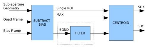
*Figure 2.2: The Bias Frame is subtracted to estimate the background. The background is also subtracted to estimate the x-y spot position.*
