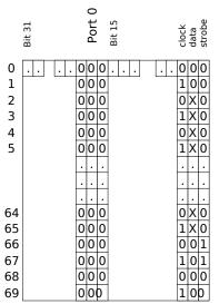
*Figure 2.4:* The number of points per channel is 35. Each point is represented by two consecutive 32 bit integers in the output buffer (one clock period).
