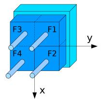
*Figure 2.3: TT probe x-y coordinate system. The convention follows the one proposed in document [7].*
