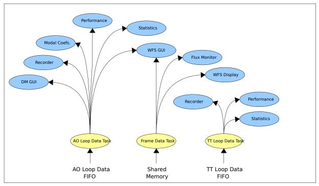
Figure 3.1: Data acquisition in RTSOFT is built using a consumer producer model.
