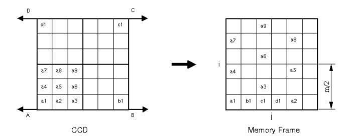
Figure 3.2: Diagram showing the scrambling of the data produced by the quad CCD readout process.
